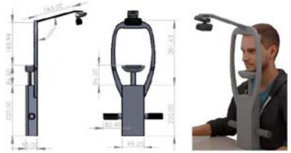
Fig.4 Engineered to mitigate motion artifacts, this 3D-printed apparatus uses an ergonomic design to comfortably immobilize the user's head and maintain a consistent viewpoint for the camera.
