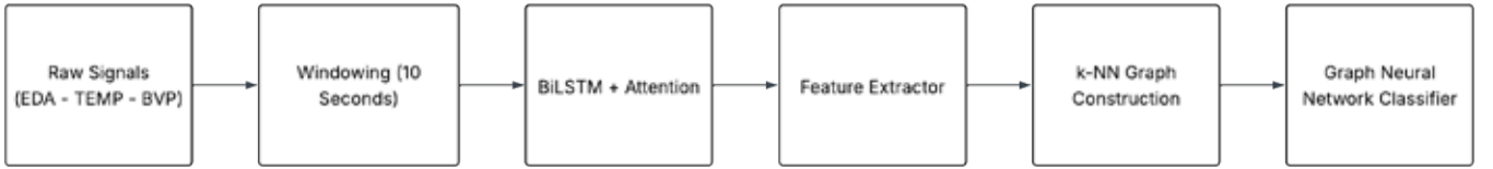
Figure 2: Overview of the proposed IA-IGNN pipeline. Raw wrist signals are segmented into 10-second windows and encoded via a BiLSTM with Attention. The resulting embeddings form a k-NN graph, which is processed by Graph Convolutional Network for baseline–stress classification.
