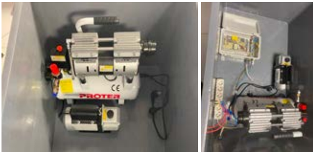
Figure 2. PROTER Air Compressor / VALUE VE-115 Vacuum Pump and Power Connections
