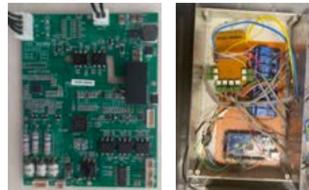
Figure 4. Arduino MEGA with 8xRelay Module and PM-4100 Vital Parameter Circuit
