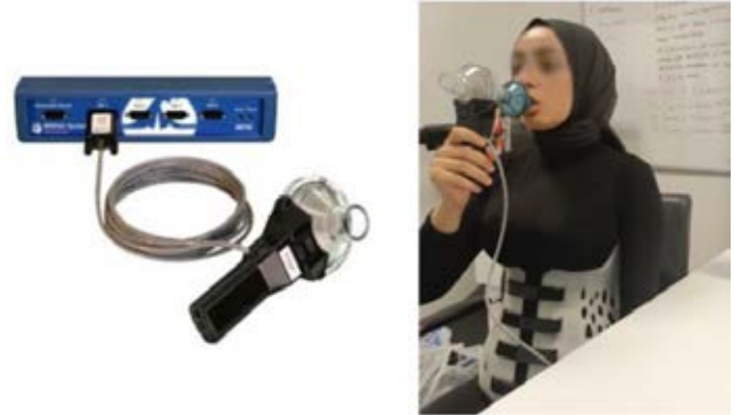
Figure 2. Experimental setup showing the BIOPAC SS11LB airflow transducer connected to the MP36 system for VC measurement during brace wear.
