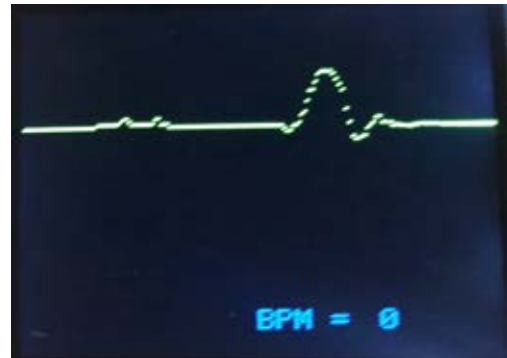
Fig. 7. Sampled ECG Result for f_s=500\text{ Hz}
