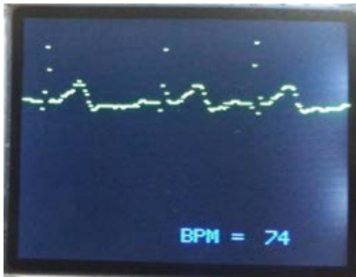
Fig. 10. Sampled ECG Result for f_s=70 Hz
