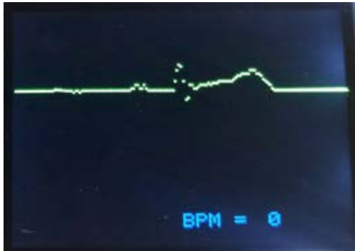
Fig. 9. Sampled ECG Result for f_s=150 Hz
