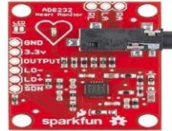
Fig. 3. AD8232 ECG Measurement Sensor [17]
