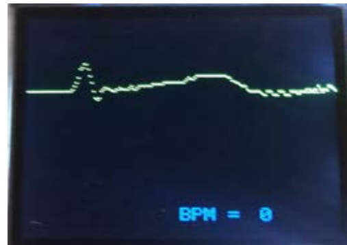
Fig. 8. Sampled ECG Result for f_s=300\text{ Hz}
