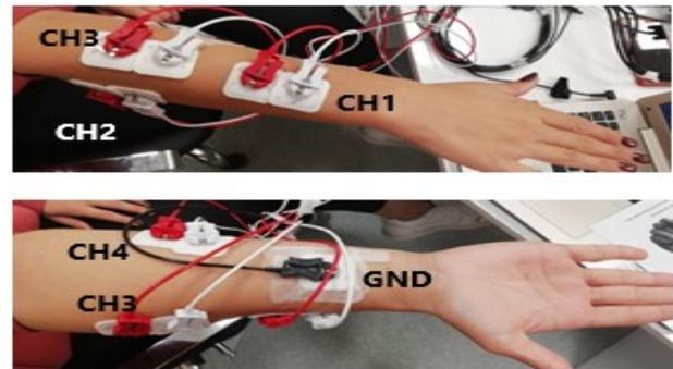
Fig. 1. Four channels of sEMG electrodes placement.
