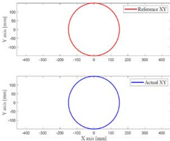
Fig. 7. Trajectory tracking performance of the robot in task space
