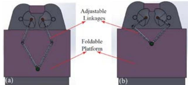
Fig. 2. Solid model of the mobile rehabilitation platform (a) Maximum allowable workspace (b) Minimum allowable workspace
