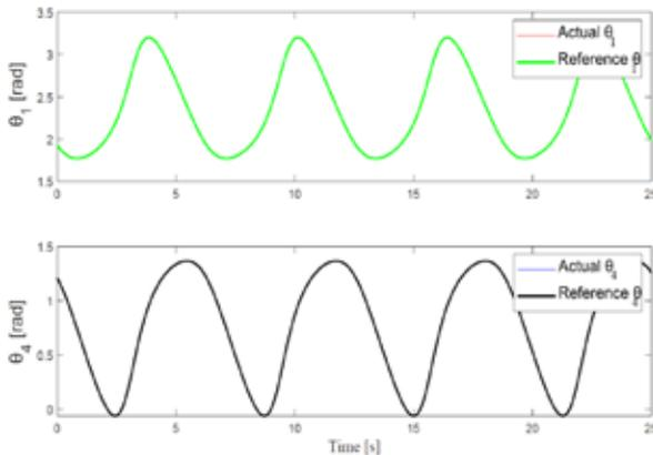
Fig. 6. Comparison of the reference and actual joint position under PI controller (a)  $\theta_1$  and (b)  $\theta_4$
