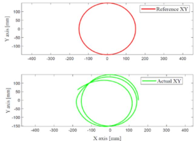
Fig. 5. Comparison of reference input (a) and actual trajectory when perturbation is applied (b)
