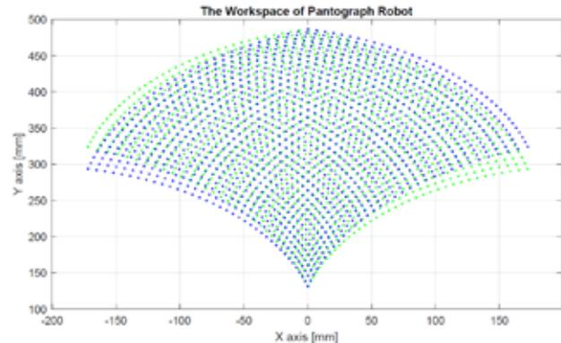
Fig. 1. The workspace of the 2DoF parallel manipulator in 2D Cartesian coordinates
