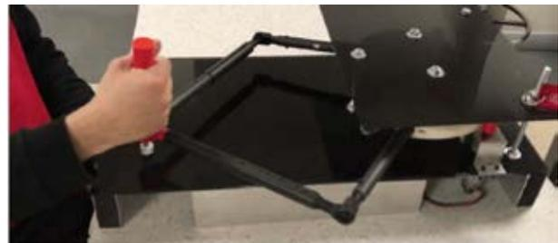
Fig. 3. The prototype of the adjustable mobile pantograph robot
