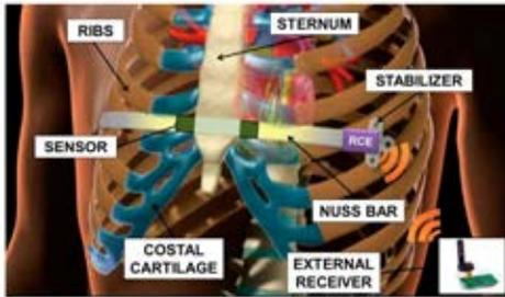
Fig. 2: Custom pectus bar equipped with sensors [8].
