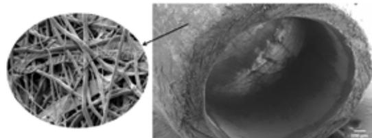
Figure 5. SEM image of fabricated microtube and PLGA nanofibers. Scale bar represents 100µm
