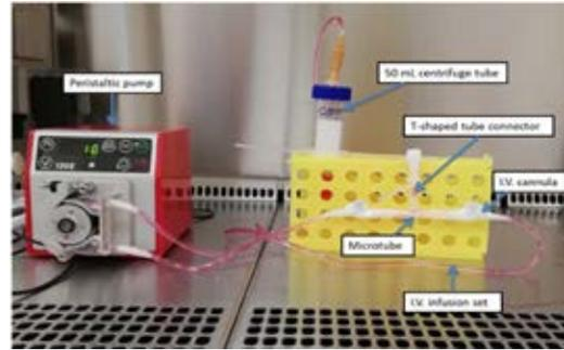
Figure 4. Bioreactor system.
