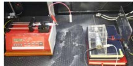
Figure 2. Electrospinning setup.
