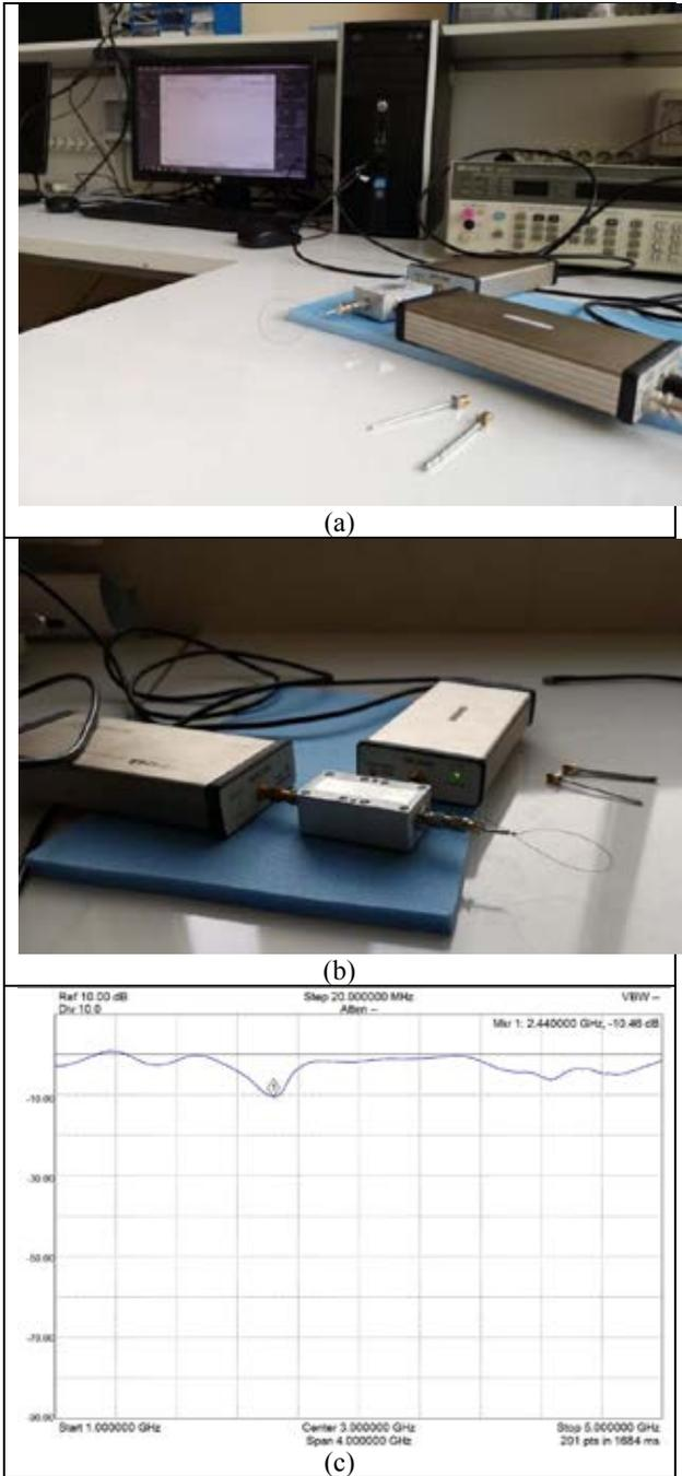
Figure 3. 2.45 GHz NiTi Ring Antenna's return loss measuring device and measurement result
