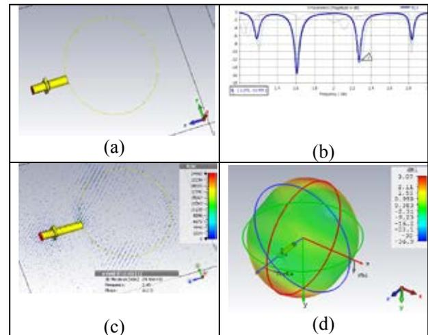
Figure 2. a) CST drawing of the NiTi Ring Antenna b)  $S_{11}$  (c) E-Field d) Directivity
