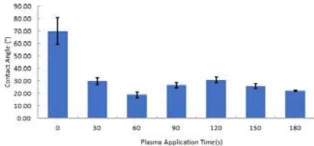
Fig.2. Contact angle change depending on plasma treatment time. Results are presented as mean  $\pm$  standard deviation.
