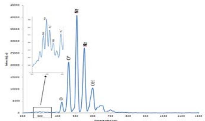
Fig.1. Optical emission spectra of air DBD plasma
