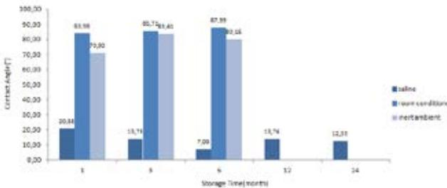
Fig.3. Contact angle measurements of 60 s plasma treated Ti discs
