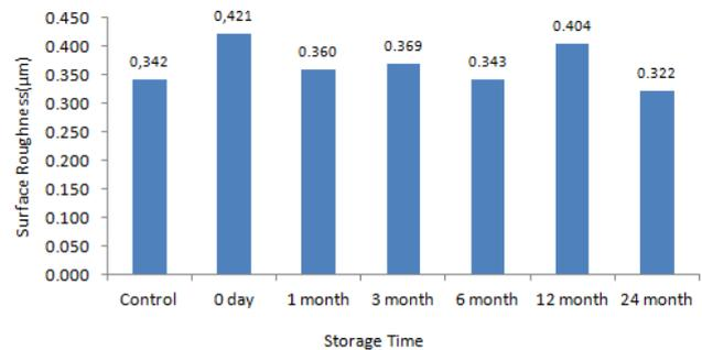
Fig.4. Storage time-dependent roughness of Ti discs in saline
