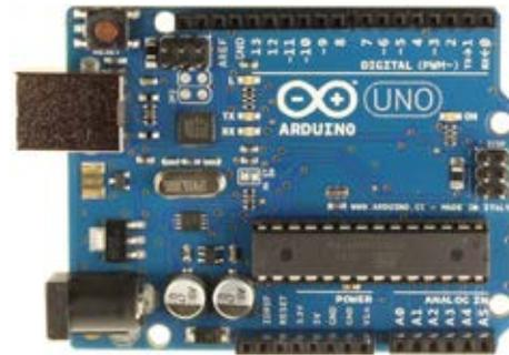
Fig. 2. Arduino/Genuino Uno R3 microcontroller
