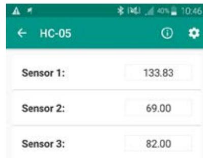
Fig. 6. Real-Time biomedical data on a smart phone. Sensor 1 represents Systolic Blood Pressure, Sensor 2 represents Diastolic Pressure and Sensor 3 represents Heart Rate.
