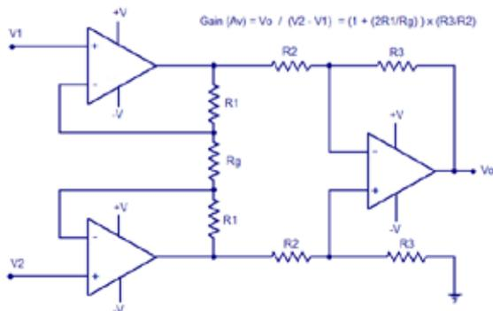
Fig. 1. Circuit diagram of instrumentation amplifier
