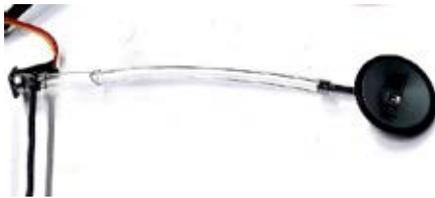
Fig. 3. Designed stethoscope for the detection of heart sounds
