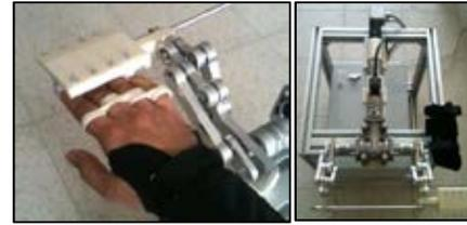
Figure. 1. a) Hand attached to the end effector of the system, b) Overall robotic rehabilitation setup [1].
