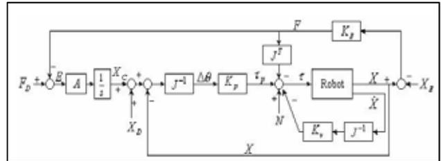
Figure 3. Admittance control block diagram [6]
