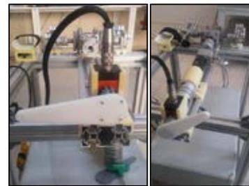
Figure. 2. a) Torque sensor calibration linkage, b) Admittance control test setup.
