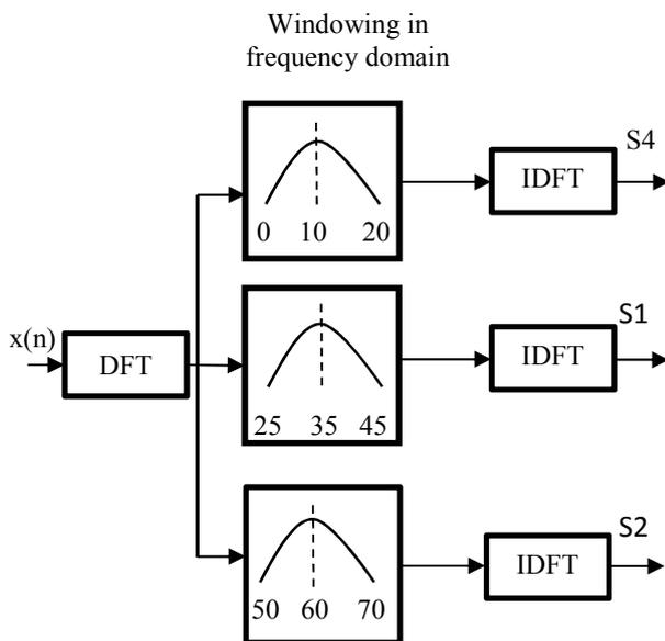
Figure 3: Decomposition of S1, S2 and S4 waves.
