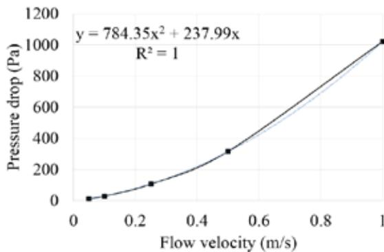
Fig. 2. Variation of pressure drop with flow velocity for 72 wires flow diverter
