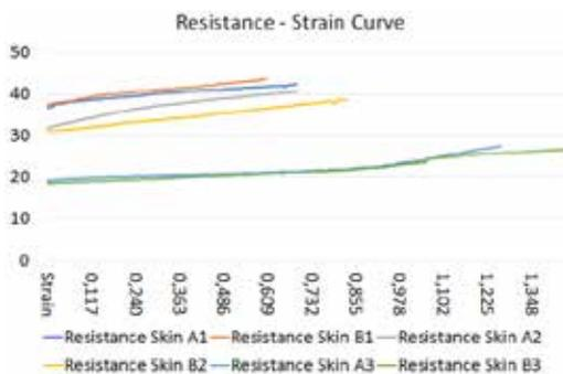
Figure 11: Resistance(kΩ) - strain curve
