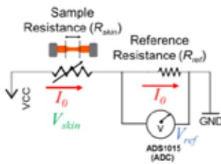
Figure 10: Electronic components diagram
