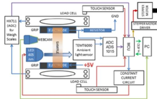
Figure 7: Electronic components diagram
