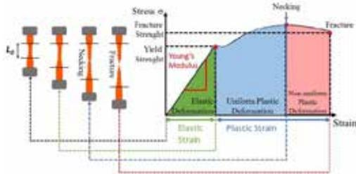
Figure 5: Tensile test result illustration: Stress-Strain Curve
