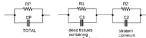
Figure 3: Equivalent circuits of skin impedance under Alternative Current
