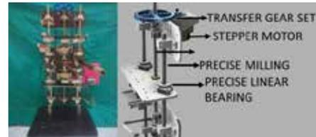
Figure 6: Mechanical parts of design
