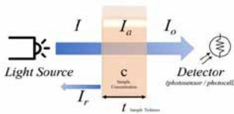
Figure 2: Light Transmittance, Absorbance and Reflection model
