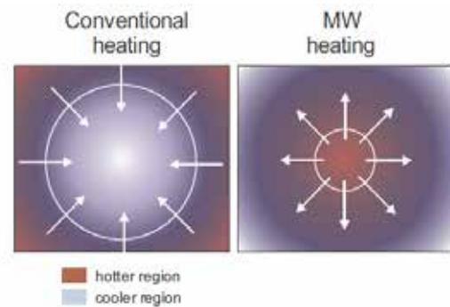
Figure 1: Temperature distribution and direction of heat transfer between conventional and MW heating. In MW heating, energy is uniformly dissipated throughout the material [8].
