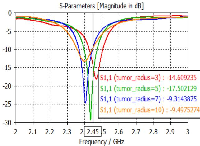
Figure 5:  $S_{11}$  parameters of microwave probe dependent on tumor dimensions
