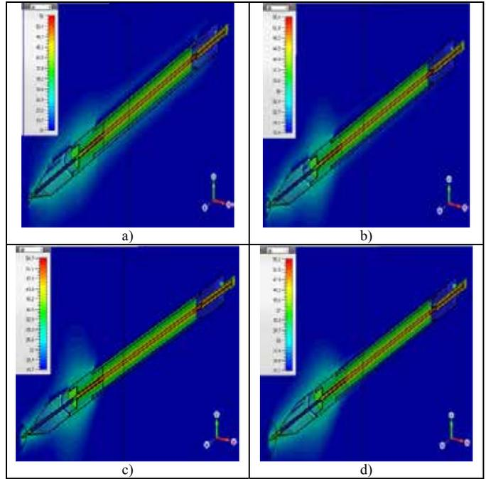
Figure 6: Radiation pattern of microwave probe dependent on tumor dimension a) Radius of tumor=3mm b) Radius of tumor=5mm c) Radius of tumor=7mm d) Radius of tumor=10mm
