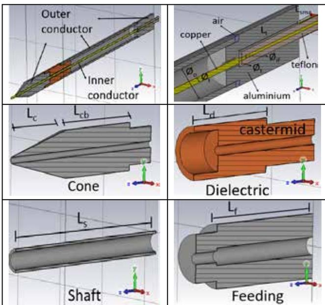
Figure 2: Microwave probe sections
