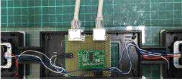
Fig. 5. Connections between HX711 and four single load cells
