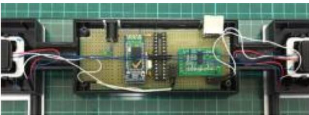
Fig. 6. Electronic circuit of the last weighing scale
