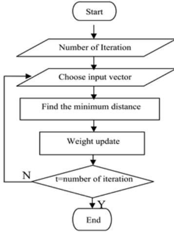
Figure 2: Flow diagram of SOM algorithm.
